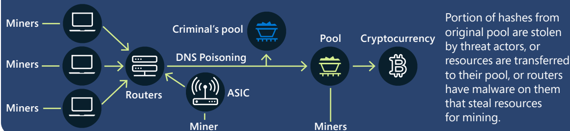
DNS poisoning of gateway devices compromises legitimate mining activities and redirects resources to criminal mining activities.
