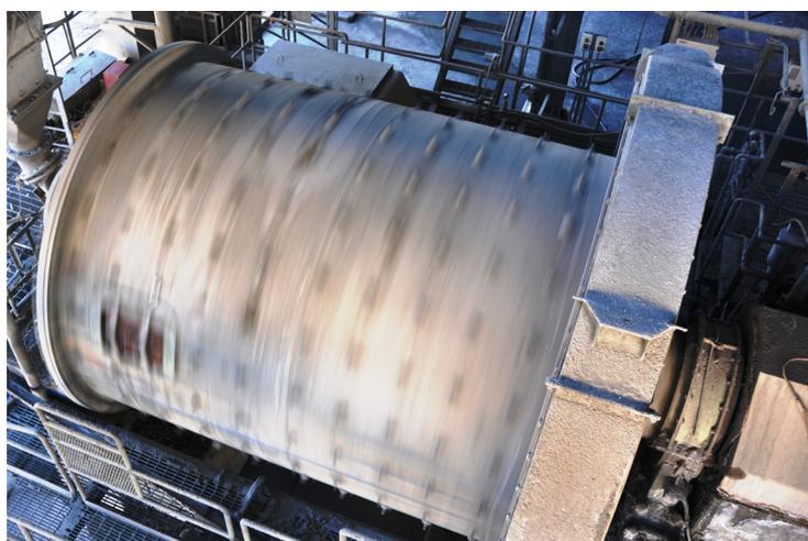
A rolling ball mill in an alumina refinery
