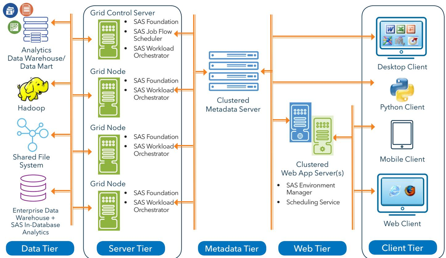
Figure 1: SAS Grid Computing architecture.
