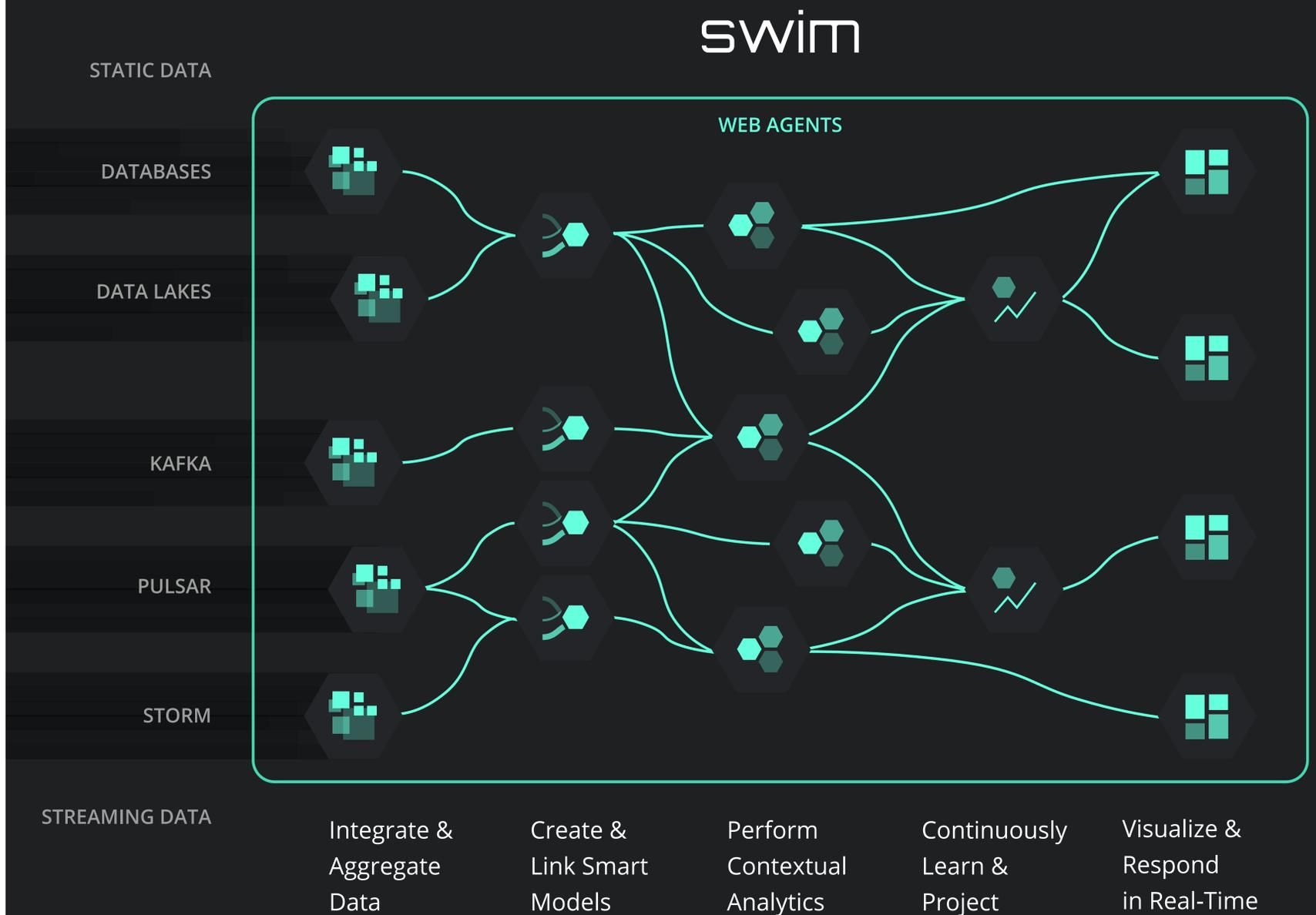
Swim Web Agents are web-scale, autonomous computer programs that aggregate, transform, analyze and act upon streaming and static data at the speed of change; they are the foundation of Swim continuous intelligence applications. Swim Web Agents are self-contained objects that possess individual logic and manage their own granular data streams and persistence.
