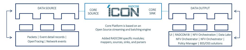
RADCOM I.C.O.N. is a single containerized, stateless component that combines front-end probe functionality with complex-back end processing into one standalone monitoring cluster delivering full network visibility in 5G from the RAN to the network core.
