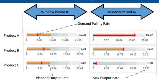
HARMONIX V-Sensor measures net output for each Product ID planned against the demand pulling rate. It also provide real-time feedback of planned output rate against your maximum net output capacity. Very useful to evaluate available capacity to meet demand in real-time at selected window period of the month.
