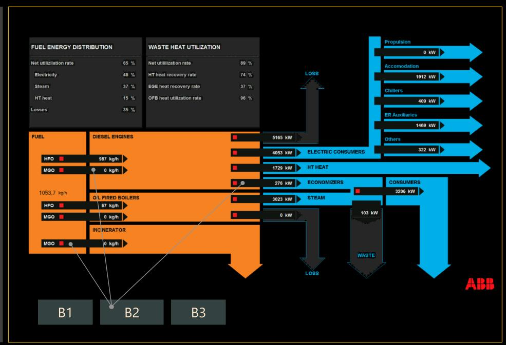
Diagramics Visual Automation Examples - Marine Control Panel
