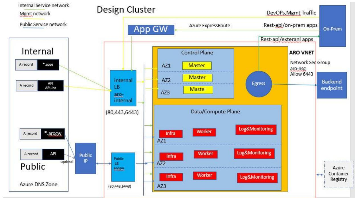
Figure: Principal Concept design for ARO Cluster (Orange area is cover by G-Able ARO Advance Package)
