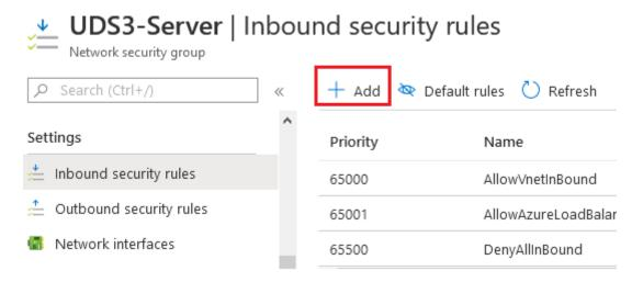
7. You will need to configure two "Network security groups": one for the UDS server and one for the UDS Tunnel server, each with its corresponding rule in "Inbound security rules". In the following table, you can check the ports necessary to access the UDS components and the service they will offer:
