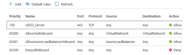
b) **UDS Tunnel:** You must create an access rule to the UDS Tunnel server where you allow traffic through 443 TCP and 10443 TCP ports:
