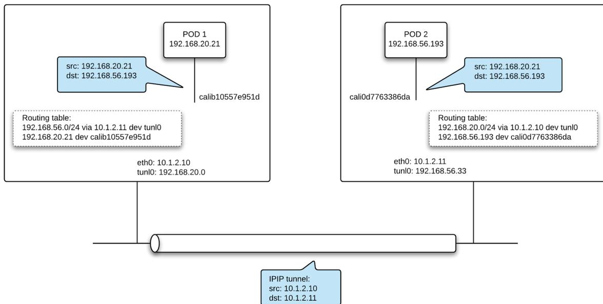
The above diagram shows how a packet traverses between pods on different nodes. In this example the Calico CNI network plugin is used. Every network plugin has a different approach for how a Pod IP address is assigned (IPAM), how iptables rules and cross-node networking are configured, and how routing information is exchanged between the nodes.
