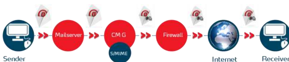
Figure 1: Process of CompuMail Gateway within network infrastructure
