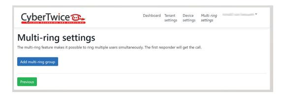
Name the Multi-ring group and add a description. The name combined with the fixed domain: cybergate.cybertwice.com will make the call destination. E.g.: If the name is TestGroup, the name to dial in the intercom will be:TestGroup@cybergate.cybertwice.com.
