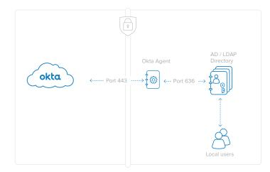
Figure 6: Okta Agent connections are Port 443 for AD (SSL Encrypted) and over Port 636 for LDAP. No firewall changes are needed for either the AD or LDAP Agents.
