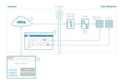
*Figure 9: Okta enables SSO for LDAP authenticated internal web applications*
