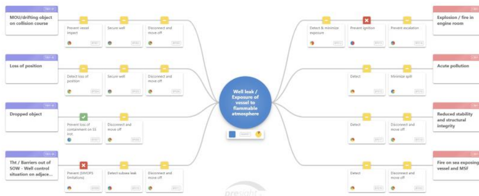
Illustration 1: The illustration shows the bowtie methodology that the solution is based on.
