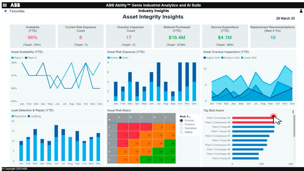
Managerial Asset Integrity Dashboard Indicating Heat Exchanger 4# As Bad Actor
