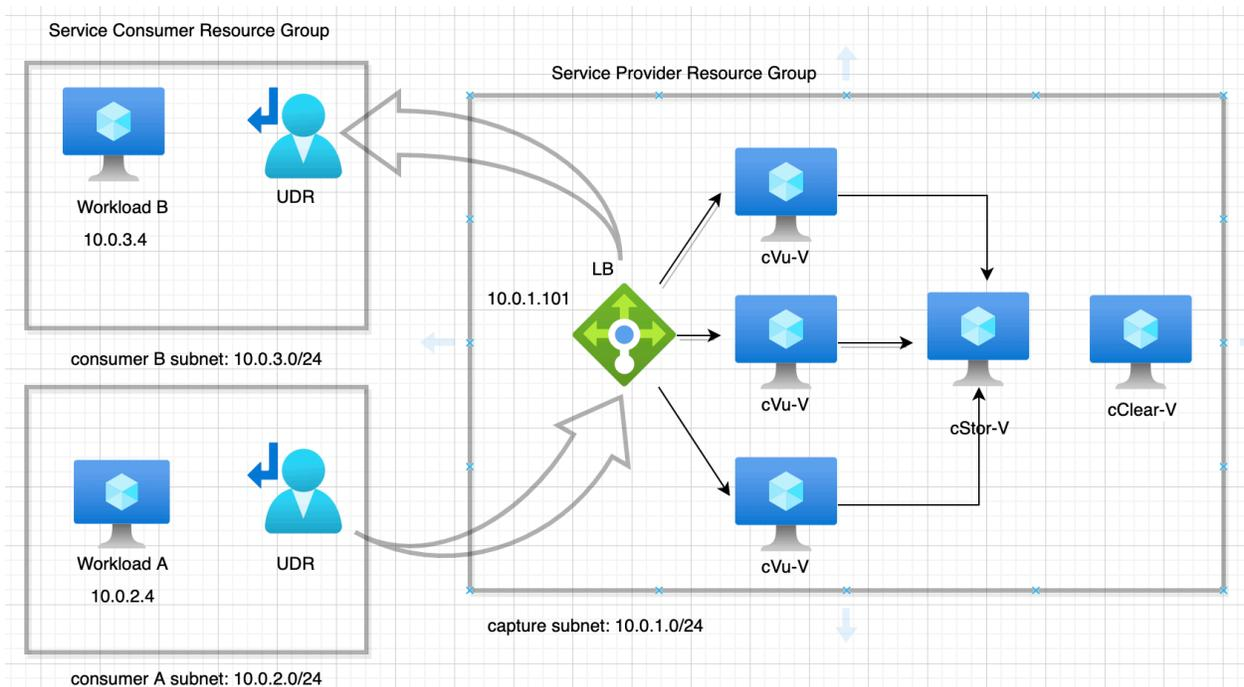
Traffic coming from the 10.0.2.0/24 subnet on the bottom left destined for the 10.0.3.0/24 subnet on the top left is going through a [User Defined Route \(UDR\)](#). That route sets the “Next Hop” to be the load balancer 10.0.1.101.
