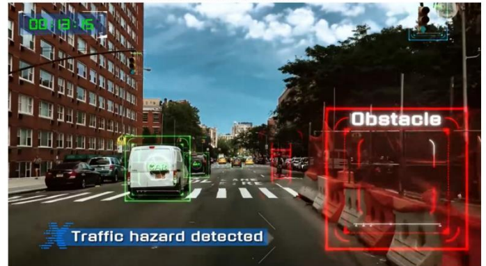
The Monitoring SaaS module also identifies traffic hazards/obstacles:
