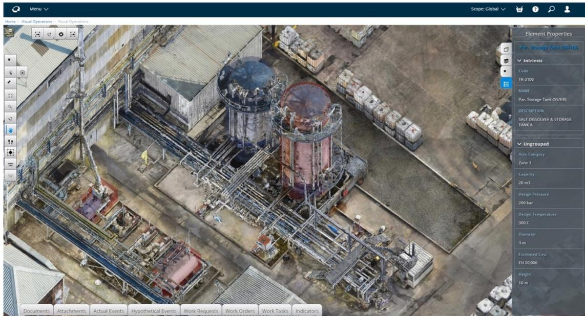
**A Reality Mesh Model with Functional Context: Highlighted Areas Are Identified Process Units with Properties (Image Courtesy of Bentley Systems)**
