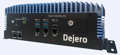
The FirstNet Ready™ GateWay 211 network aggregation device provides reliable connectivity to the Internet, cloud applications, and private networks. The ruggedized and fanless chassis is ideal for installation in vehicles and portable kits.
