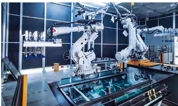
Vision-Guided Window Glass Gluing
