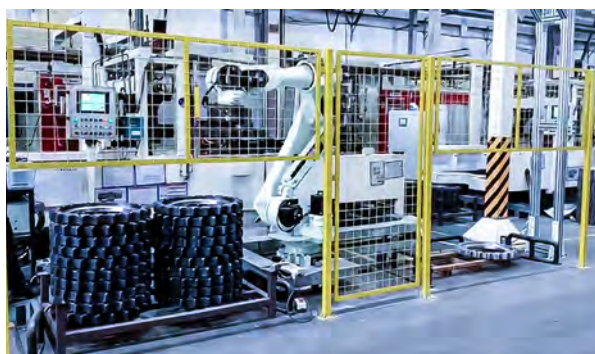
Vision-Guided Machine Tending of Drive Gears
