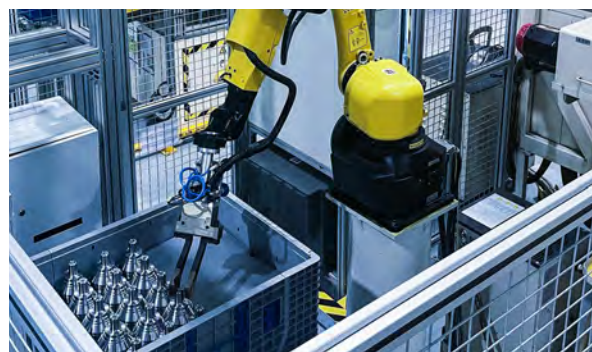
Vision-Guided Bin Picking of CV Joints
