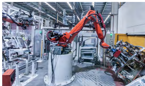
Vision-Guided Car Door Inner Panel Picking
