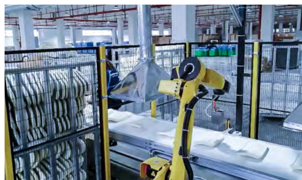
Vision-Guided Gluing of Seat Backs
