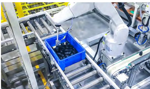
Vision-Guided Bin Picking of AC Foot Pads
