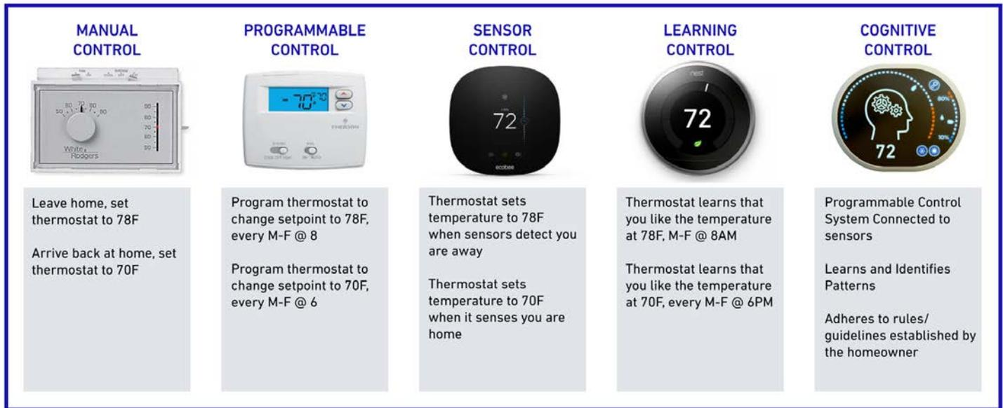
Figure 11. Example of evolution from manual control to cognitive control
