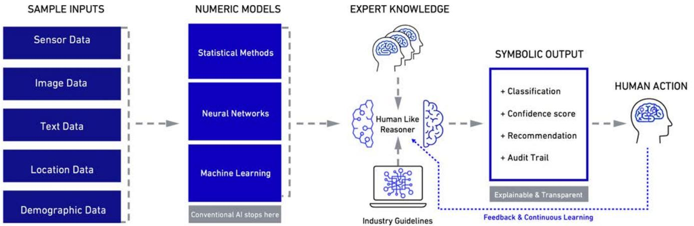
Figure 5. Beyond Limits LUMINAI™ Cognitive Reasoner high-level architecture
