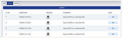
Color analysis (Grading mix of coal) in real-time and automated alerts for any deviation from ideal profile for immediate redressal by the plant operators
