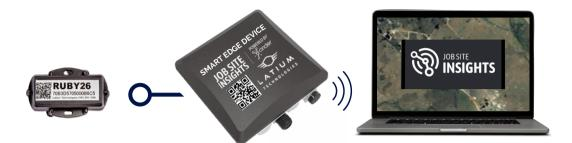
The sensor monitors the asset and sends all adverse alerts to the Smart Edge Device which then translates the data into the Job Sight Insights platform for convenient user viewing.
