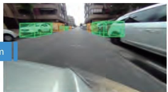
**Data Annotation** HelloData AUTO starts vehicle detection after smoothing distortions of the fish-eye lens by applying Geometric Rectification technique
