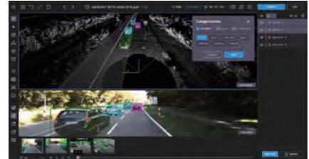
3D Lane Detection using Cuboid in LiDAR Data
