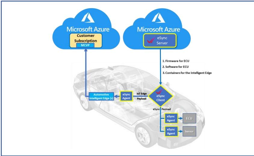
The Excelfore eSync OTA pipeline is how MCVP customers will be able to deploy updates to their fleets of vehicles, whether those updates are firmware to ECU's or containers for Automotive Intelligent Edge (Microsoft IoT Edge-based runtime environment).
