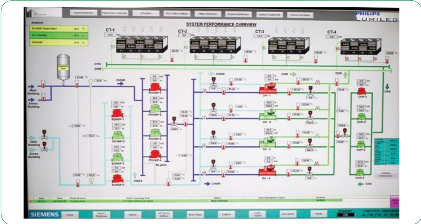
The chiller plant management system enables the required cooling to be delivered in an energy-efficient manner.
