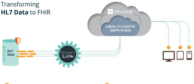
As it travels through the SmartLink<sup>tm</sup> system, it is transformed into **FHIR** objects
