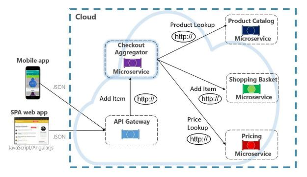
Figure 4-10. Aggregator microservice
