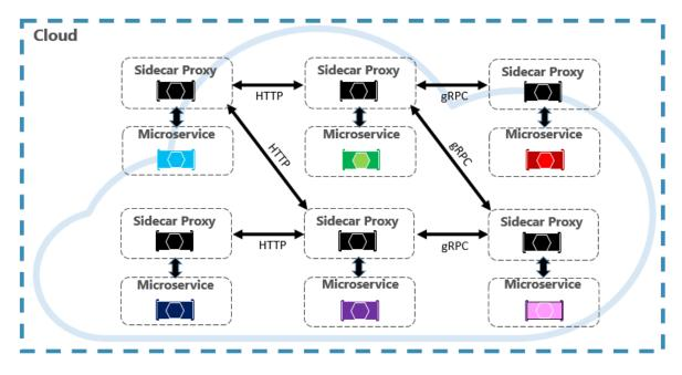
Figure 6-7. Service mesh with a side car
