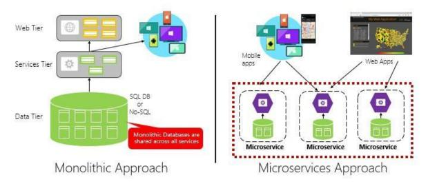
Figure 1-4. Monolithic versus microservices architecture
