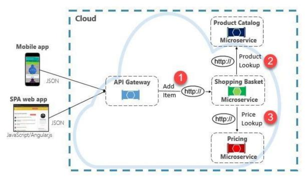
Figure 4-8. Direct HTTP communication While direct HTTP calls between microservices are relatively
