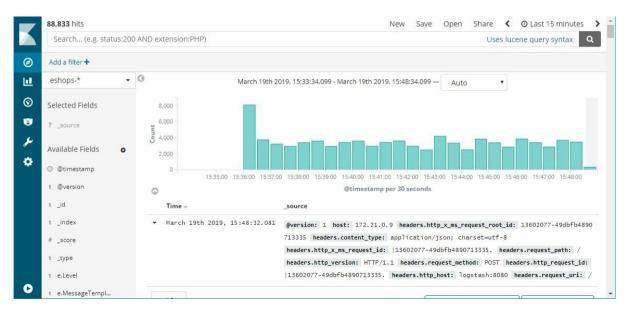
Figure 7-6. An example of a Kibana dashboard showing the results of a query against logs that are ingested from Kubernetes
