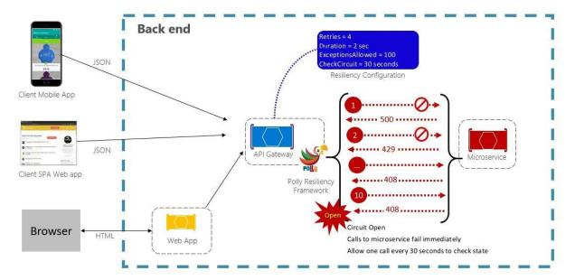
Figure 6-3. Circuit breaker pattern in action
