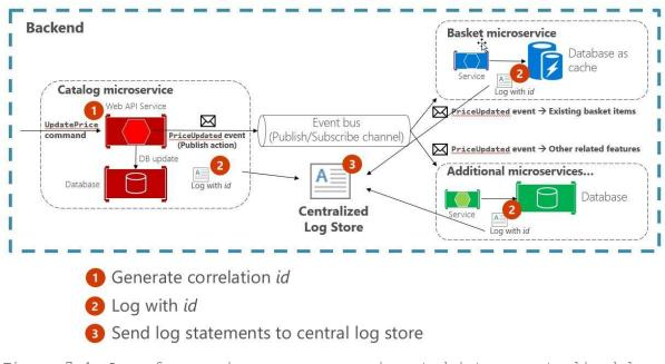
Figure 7-4. Logs from various sources are ingested into a centralized log store.
