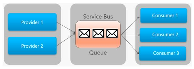
Figure 4-14 outlines the high-level architecture of a Service Bus queue.
