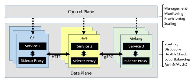
Figure 6-8. Service mesh control and data plane
