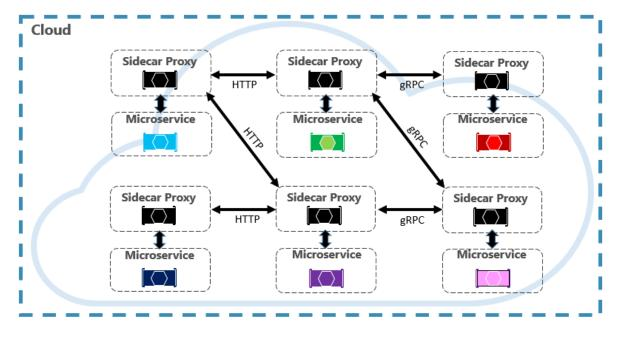
Figure 4-24. Service mesh with a side car
