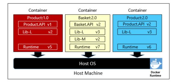
Figure 1-6. Multiple containers running on a container host
