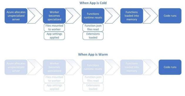
Figure 3-9 shows a cold-start pattern. Note the extra steps required when the app is cold.
