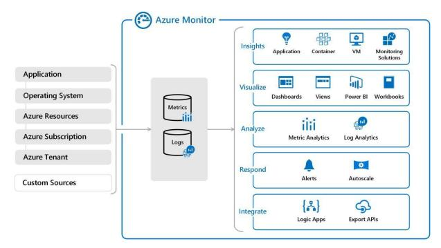
Figure 7-12. High-level view of Azure Monitor.
