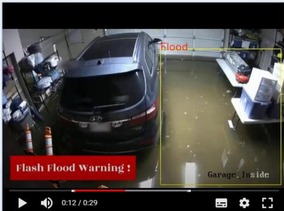
AI will detect flood by capturing glossy of surfaces and calculate as a percentage of total area. If it exceed the setting, system will alert to relevant team
