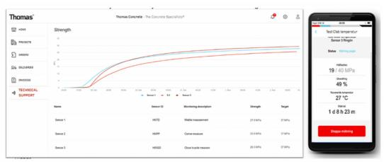
Thanks to this service, there's no need for Thomas customers to be on-site to check the status of the concrete curing. They can instead monitor the process remotely, using the online portal or the mobile app
