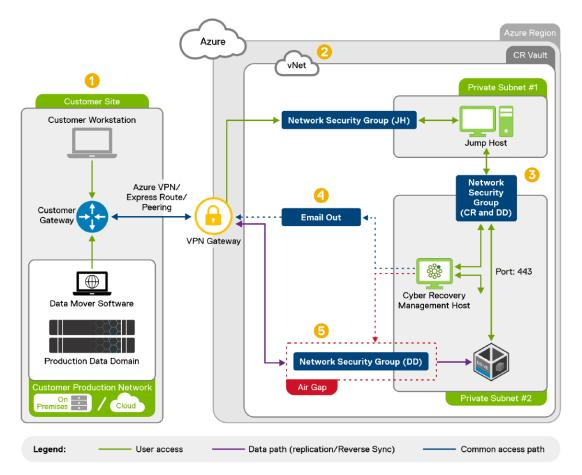
1. The production environment can be on premises or also deployed on Azure. The workstation at the production site enables you to connect to the jump host, which is in a private subnet in the VNet. The jump host provides access to the Cyber Recovery management host and the DDVE management console. For additional security, the workstation has a limited IP range.
