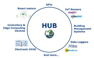
Like the Data Communication Company, which connects smart meters to suppliers in the gas and electricity industry, the ARM Hub is a connector to the district energy industry's smart meters, building management systems, connected controllers and more.
