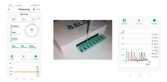
ATTENTION, if the lines on the chart do not appear after pressing the start button do not add the sample. Stop the measurement and start it again. Ensure that the lines are visible in the chart and they all start at 0 mV before adding the sample. In case lines do not start at 0 mV stop the measurment and start it again.
