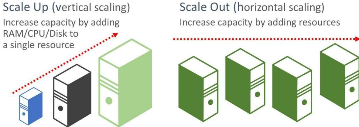
Figure 6-6. Scale up versus scale out
