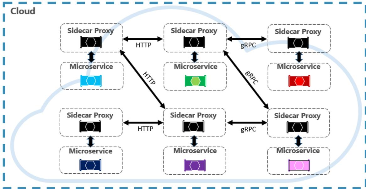
Figure 4-24. Service mesh with a side car
