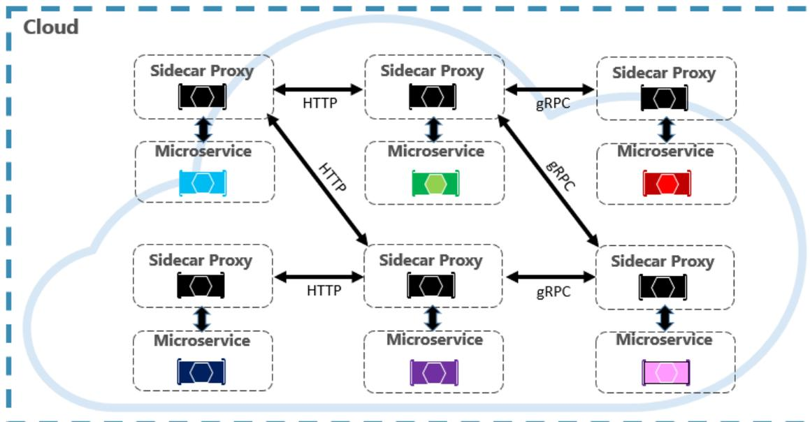
Figure 6-7. Service mesh with a side car
