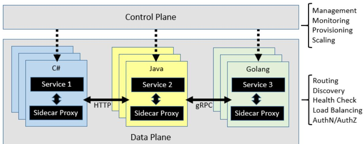
Figure 6-8. Service mesh control and data plane
