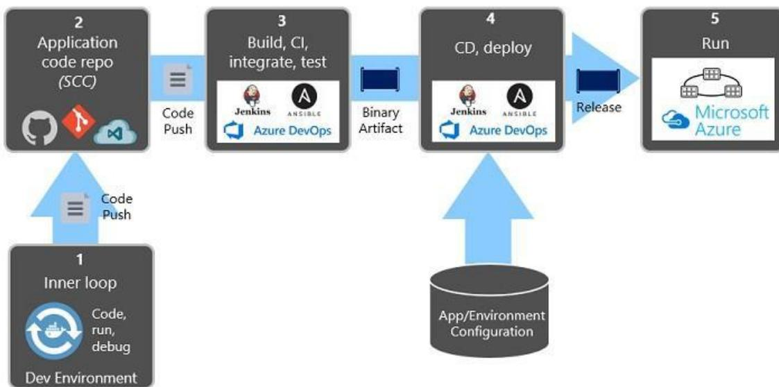
Figure 1-9. Deployment steps in a CI/CD Pipeline
