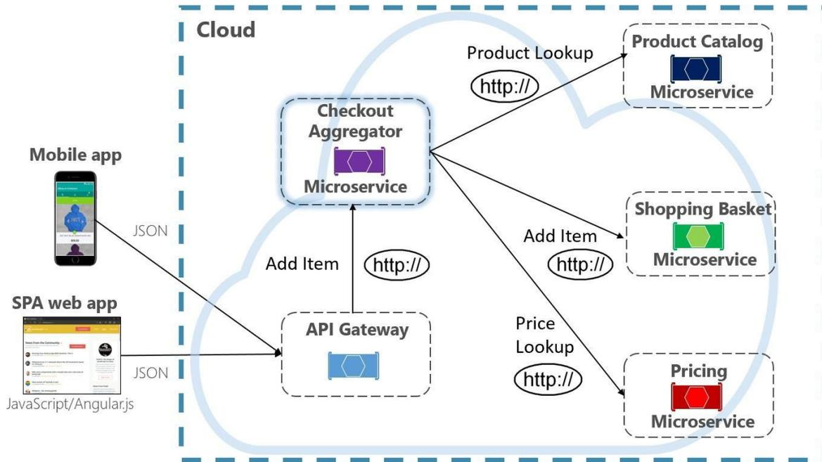
Figure 4-10. Aggregator microservice
