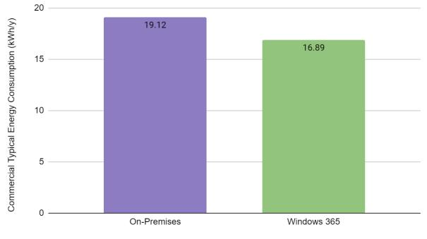
Figure 2. Notebook computer electricity consumption (kWh) for on-premises and Windows 365 operations
