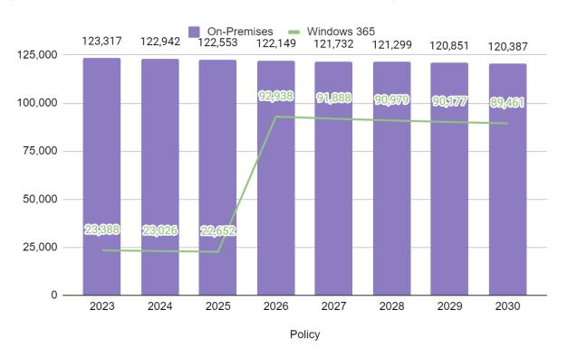
Figure 11. Total annual end user computing device carbon footprint (kgCO<sub>2</sub>e) by policy
