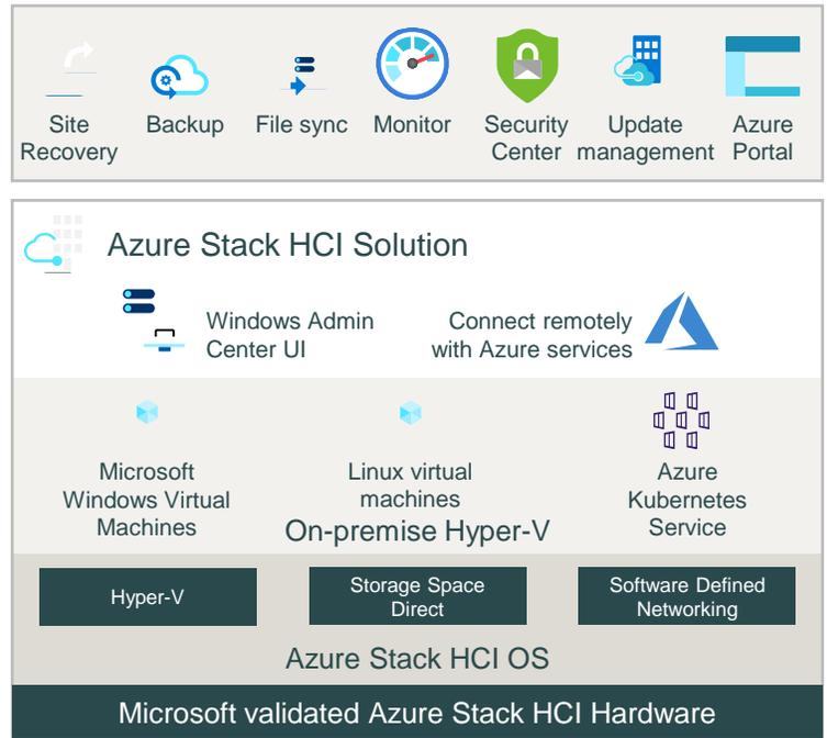
Figure 2. Azure Stack HCI implementation, technical components
