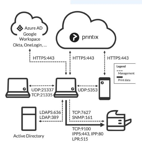
Figure 2: Overview over ports and network protocols used in Printix.
