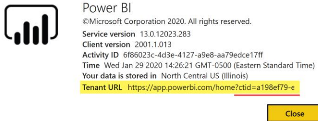
Figure 62 - The ctid is available in the Tenant URL under the Help > About menu
