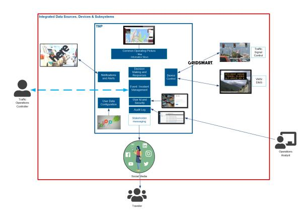
In the example above, core TMP capability is shown by the blue box. The surrounding red box shows the connected data sources, devices and subsystems that TMP has integrated with. For example, live congestion data from HERE is being displayed on the map based common operational picture. There are also GRIDSMART cameras providing data and images to TMP operators.
