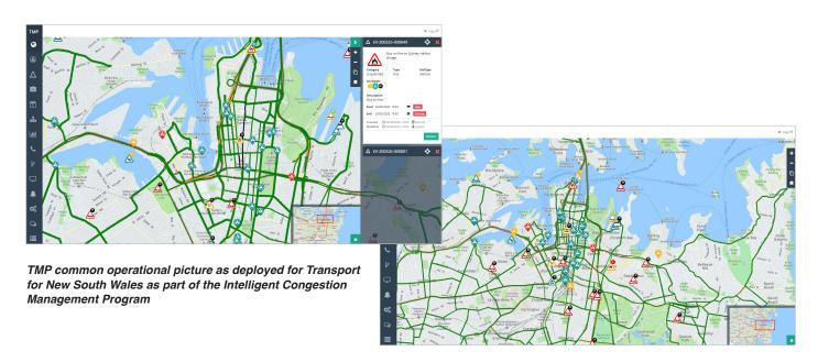
Key to the COP is the range of information available to the operator through the COP display. All connected roadside devices, traffic conditions, public transport information and other available data sources are all displayed. All future technologies and data feeds will continue to be integrated into the COP, supporting the paradigm of a single operational management system.
