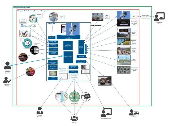
In this example, automatic number plate recognition cameras are integrated into TMP. Along with the other roadside infrastructure, they are controlled and managed through TMP. However, the offence processing is done though a separate specialist offence processing solution which is integrated with TMP.
