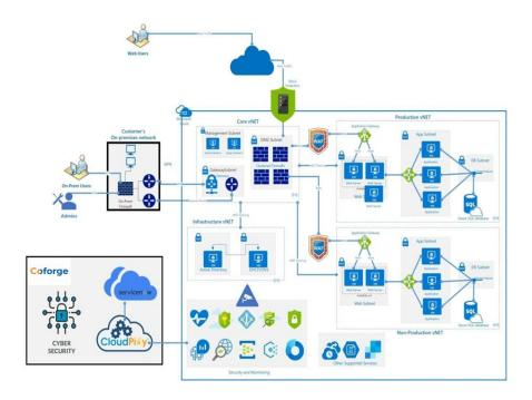
This architecture also integrates security monitoring and policy management across Azure subscriptions, and prevent, detect, and respond to threats with increased visibility into and control over the security of resources through Azure Security Centre. Enforcing intelligent azure access policies to the solution, helps cloud environment become compliant with internal policies and external regulations.
