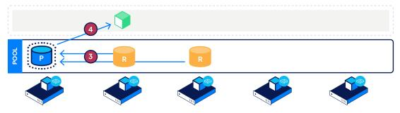
**5/6.** If a node fails, a replica is automatically promoted to become a new master and another replica is provisioned on an available node. Volume mount points move transparently to the application.
