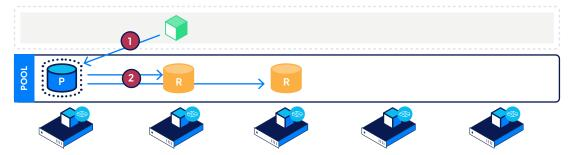
3/4. All acks need to be received by the primary and the write needs to be acknowledged to the application.
