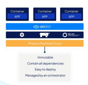
To run applications which require persist storage within containers, we require a layer which can provide persistent disk storage to those containers, independent of the lifecycle of the containers themselves.
