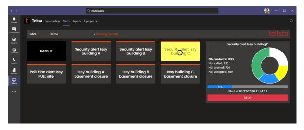
The alert may be triggered by calling a directory number, from an authorized calling number and eventually by typing a DTMF code. The alert is selected according to the number dialed (one number per alert), or according to a list of calling numbers. A DTMF code may be also required to trigger the alert.
