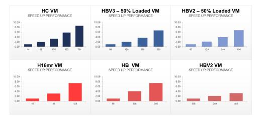
Figure 4 : 2020R2/2021R2 Mechanical Direct Solver shows strong scale up for 16 million DOF Highly Nonlinear Problem
