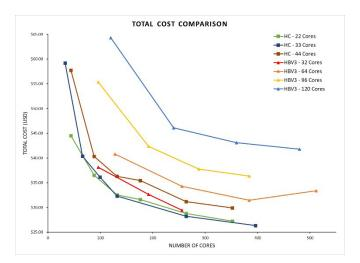
Figure 6.3: 2021R2 Mechanical Direct Solver performance comparison between HC and HBV3 –Total Cost Focused
