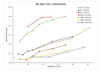
Figure 6.2: 2021R2 Mechanical Direct Solver performance comparison between HC and HBV3 –HW Cost Focused
