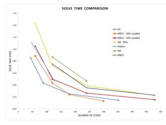
Figure 5: 2020R2 Mechanical Direct Solver performance across different VM Configurations
