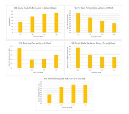
Figure 13: Example HB performance metrics for Fluent.
