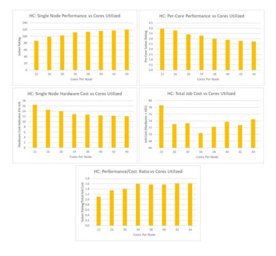
Figure 15: Example HC performance metrics for Fluent.
