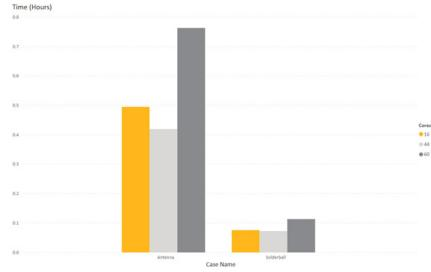
Figure 9 compares solution times for two HFSS models on the 16-core H16mr, 44-core HC, and 60-core HB.
