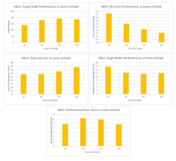
Figure 14: Example HBv2 performance metrics for Fluent.
