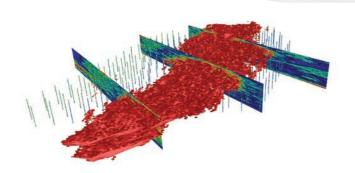
Quickly discern ore and waste rock and high and low grade.
