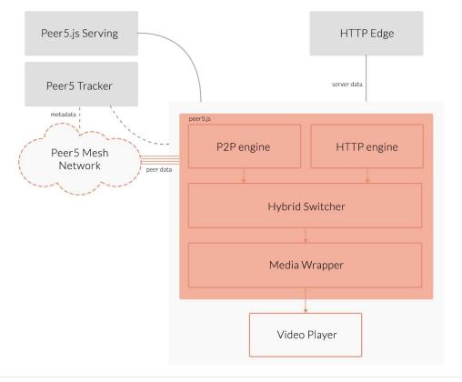
With Peer5 deployed, users can fetch chunks from the HTTP Edge and/or the P2P Mesh Network
