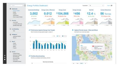
Figure 1. C3 Energy Management provides facility managers with a real-time dashboard to monitor portfolio energy usage and expenditure
