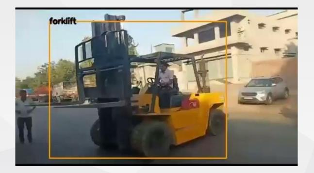
If there is a human around forklift and tractor that is working, system will alert to assigned team to take an action immediately to prevent the accidents
