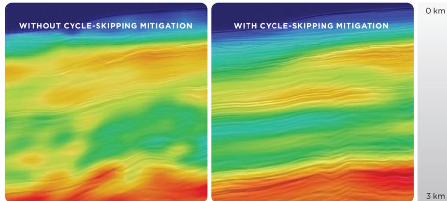
**ABOVE:** The phenomenon of cycle-skipping can result in inaccurate velocity models and poor imaging (left). Cycle-skipping mitigation overcomes this problem delivering accurate results (right) even from very simple starting models.
