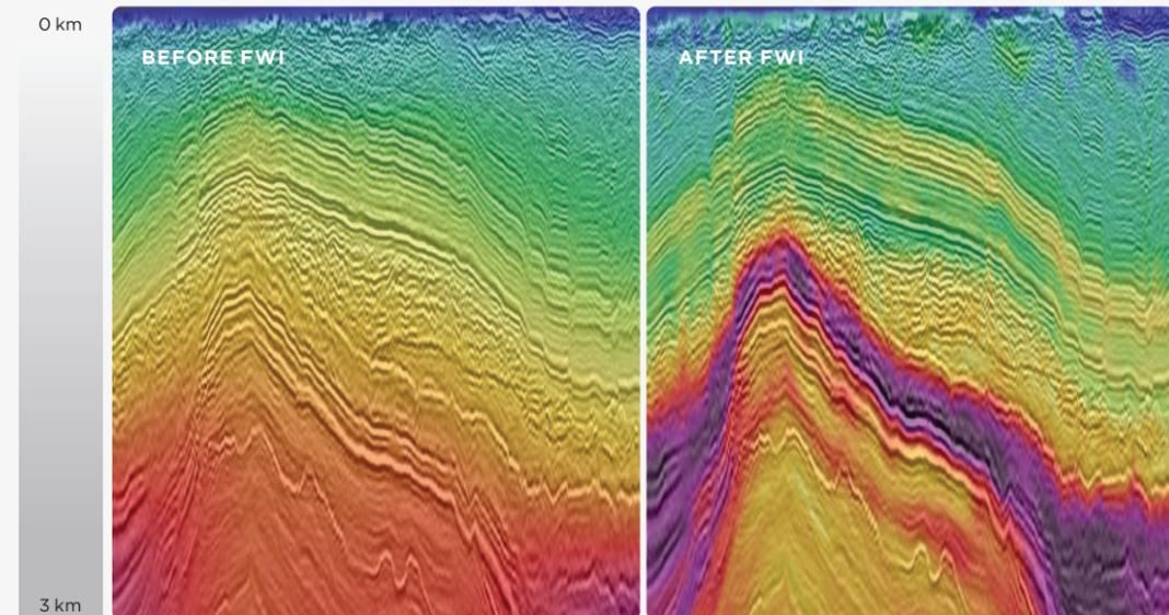
**LEFT:** This onshore vibroseis survey had favourable low frequencies, long offsets and full azimuth. However, the lack of offset in shallow resulted in the poor imaging of the overburden and the degradation of imaging quality at depth. **RIGHT:** After FWI there are noticeable improvements throughout the section – with opportunity for interpretation of the near surface, improved imaging of events at all levels and better definition of a high velocity layer.
