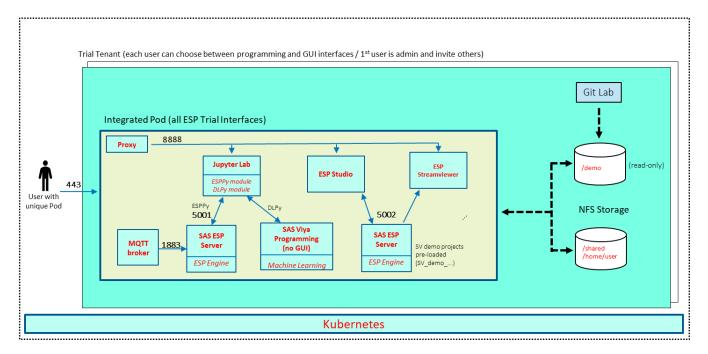
As shown in the diagram, the environment has several containers in each pod communicating with each other using predefined ports, and all communication to the external world is done through the standard port 443 to ensure that there are no conflicts with firewalls on the user side -- providing a secure environment.
