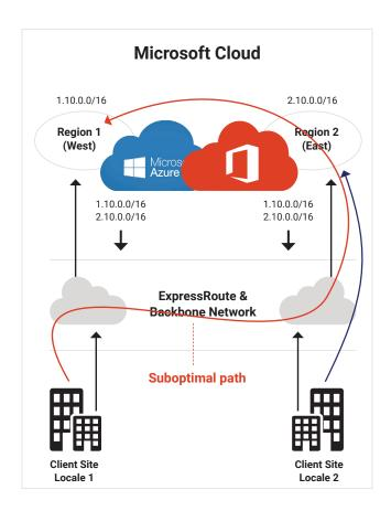
Two different client locales connecting to Microsoft Cloud. Due to the way routes are advertised, client locale 1 is using a **suboptimal** path to reach its closest Microsoft Cloud node
